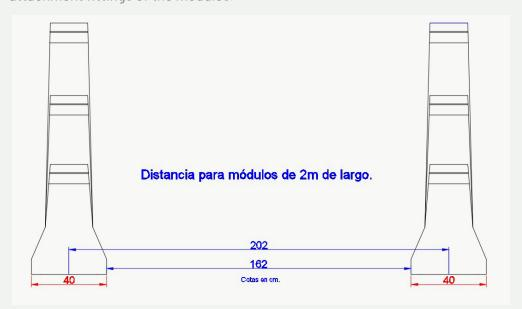
The separation among SOLARBLOC $^{\circ}$  H-S/18 structures will be different depending on the module proportions.
