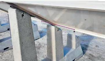
SOLARBLOC® H-S accepts a height difference among supporting plans of 4% the length of the module, with no need to level the attachment fittings of the modules.
